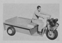
Smithco, Inc., introduces the Ranger-23, an enlarged model of the Red Rider mobile work cart, but with extra features. The three seat vehicle has a rated capacity of 23 cubic feet, a heavy-gauge steel ramp loading tailgate. The carrier floor is 8 inches from the ground. Powered by an 8hp engine, cart runs on a friction clutch.
