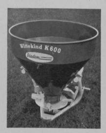
Vandermolen Export Company introduces the Diadem Fertilizer Spreader, model K600, which features a 1,600-pound capacity conical hopper. It also has a centrifugal spinner capable of spreading powder, seeds and granular fertilizer in a 50-foot swath. The width of the spread can be set from 3 to 32 feet. Coverage can be regulated from 4 pounds to 2,600 pounds
