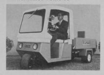
E-Z-Go Car Division offers the GT-7 truck, which has as standard equipment, double seats with back rests, automotive steering, corrosive resistant dump body, trailer hitch, dual headlights, oil pressure indicator and fuel gauge. Optionals include a ramp loader, spray boom, seed spreader and fiberglass cab.
