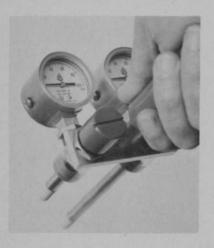
Soilmoisture Equipment Corp. announces the Turf-Probe, which measures at two levels soil moisture for plant growth. The readings are in centibars of soil suction and are independent of soil type, temperature or salinity. The unit is self-contained, requires no batteries, adjustments or calibrations and consists of probe, coring tool and stand. All parts are corrosion proof; the gauges are hermetically sealed. Parts and workmanship are guaranteed for one year. Price: \$90 f.o.b. Santa Barbara.
