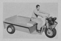
Smithco, Inc., introduces the Ranger-23, an enlarged model of the Red Rider mobile work cart, but with extra features. The three seat vehicle has a rated capacity of 23 cubic feet, a heavy-gauge steel ramp loading tailgate. The carrier floor is 8 inches from the ground. Powered by an 8hp engine, cart runs on a friction clutch.
