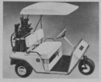
**E-Z-Go Car Division** is showing threeand four-wheel (models X-440, X-444) electric golf cars. The cars measure 90 inches long, 47 inches wide, 45 inches high and have a loading capacity of 800 pounds. The frame is rectangular steel tubing; the body is constructed of steel panels, and the seats are foam rubber over wrapped
