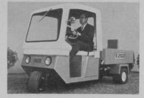
**E-Z-Go Car Division** offers the GT-7 truck, which has as standard equipment, double seats with back rests, automotive steering, corrosive resistant dump body, trailer hitch, dual headlights, oil pressure indicator and fuel gauge. Optionals include a ramp loader, spray boom, seed spreader and fiberglass cab.
