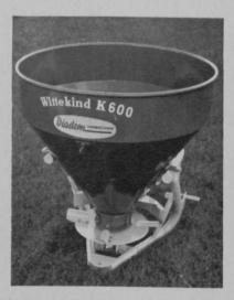
Vandermolen Export Company introduces the Diadem Fertilizer Spreader, model K600, which features a 1,600pound capacity conical hopper. It also has a centrifugal spinner capable of spreading powder, seeds and granular fertilizer in a 50-foot swath. The width of the spread can be set from 3 to 32 feet. Coverage can be regulated from 4 pounds to 2,600 pounds Continued on page 106
