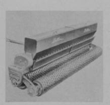
Brillion Iron Works, Inc., introduces a turf seeder, which uses fluted feed rolls to crush, seed and roll in one operation. The seeder can be adjusted to suit varying job requirements, including fine seeding. Turf-Maker comes in 8- and 10-foot drawbar models, with 6 1/8-bushel and 7<sup>1</sup>/<sub>2</sub>bushel capacity double compartment
