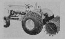
**Dedoes Industries, Inc.,** makes the Dedoes Aerator, a cylindrical unit studded with plugger tubes which can remove 296 soil plugs a revolution. Plugger tubes are made of steel, and each unit is sold with a one-year guaranteed against all mechanical defects.
