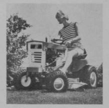
Simplicity Mfg. Company adds a new 7hp Broadmoor tractor to its line. Designed with Floating Traction tires, which according to the company leave lawns unmarked, the tractor features controlled traction differential, electric starter, adjustable bucket seats, combination brake and clutch pedal and a dash board with grouped controls.
