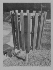
Victor Stanley, Inc., manufactures the Litter King, a trash receptacle. The frame is made of reinforced, unitized horizontal steel rings and vertical steel struts with walnut stained cypress wood slats. Each unit includes a 22 gallon plastic container.
