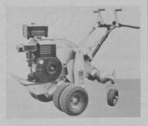
Sod-Master manufactures a turf aerating machine called Sub-Air. New features include a larger engine, heavier gear case, swiveled rear wheels and improved controls. Three parallel mounted blades at the rear of the machine penetrate seven inches below the turf; the oscillating blade movement produces a tilling action which, according to the manufacturer, loosens the sub-soil to permit deeper penetration of moisture, oxygen and fertilizer below the thatch.
