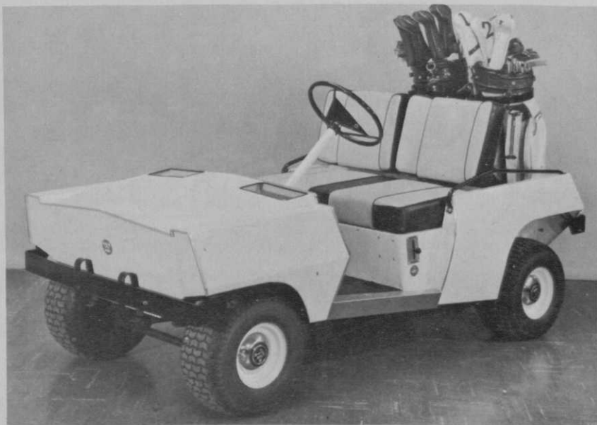
Above, Westinghouse's Marketeer 434 electric golf car with Electro-Flo speed control. It features oversize pneumatic tires that make for smoother riding.
