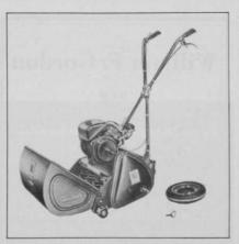
**Ransomes, Sims & Jefferies Ltd.,** has recently designed a new greens mower. The 20 inch Auto-Certes machine has a 4-cycle engine. A back-lapping attachment is available to enable the direction of the reel to be reversed for automatic sharpening.
