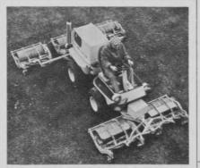
Bolens Division, FMC Corporation, recently announced that its 18 hp grounds maintenance vehicle, the GK, now utilizes a specially designed three or five gang mower for faster, more efficient reel mowing operations. The gang reels available are Roseman hollow roller-drive or laminated tire-drive tractor mounted mowers.
