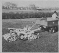
Roseman Mower Corporation has developed a new hydraulic transport Lo-Cut mower, designed primarily for mowing trees and collars or aprons around greens. The high speed, 10 blade reel gives a one-half inch frequency of cut, with a low setting height of three-eighths inch.
