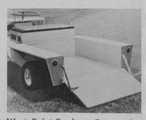
West Point Products Corporation has come out with its new Mini-Truck (R) grounds maintenance personnel/cargo carrier vehicle. It was designed specifically for grounds maintenance crews providing 16 cubic feet of cargo space. It features one-man ramp tail-gate loading.
