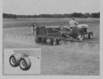
H. D. Hudson Manufacturing Company now has a tandem wheel set for power sprayers, designed to prevent wheel marks on the turf. The set distributes and spreads the weight of the sprayer over a wide area, thus carrying the load on top of the turf. The sets are available separately or as original equipment on either 100, 150 or 200 gallon sprayers or sprayer trailers.
