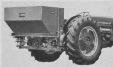
MODEL 413 "PIGGYBACK"—15 cu. ft. capacity. All the features of the 411 BROADCASTER. Attached to tractor by simple 3-point hook-up. Three-point hitch adapters available for all tractors.
