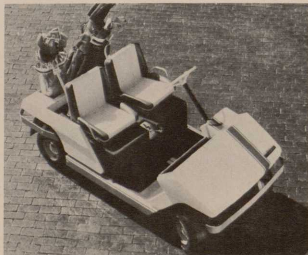
Above, the new Gran Cushman, available in both gas and electric models. It features heavy wall steel frame, and individual sports car style bucket seats.
