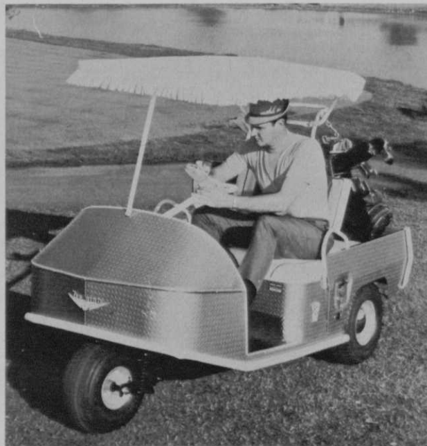
Above, Taylor-Dunn's new electric golf car. The Tee-Bird features tiller or wheel steering, six 170 amp hour electric vehicle batteries, mechanical brakes and a wide choice of colors.
