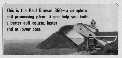
It can process up to 100 cu. yds. of soil mix in an hour. Raw materials in one end—clean, easy-to-work amended soil mixes out the other (mixes that speed grading and seeding). It features a patented highspeed cleated-belt mechanism that delivers a 5-step soil preparation that is continuous and thorough.
