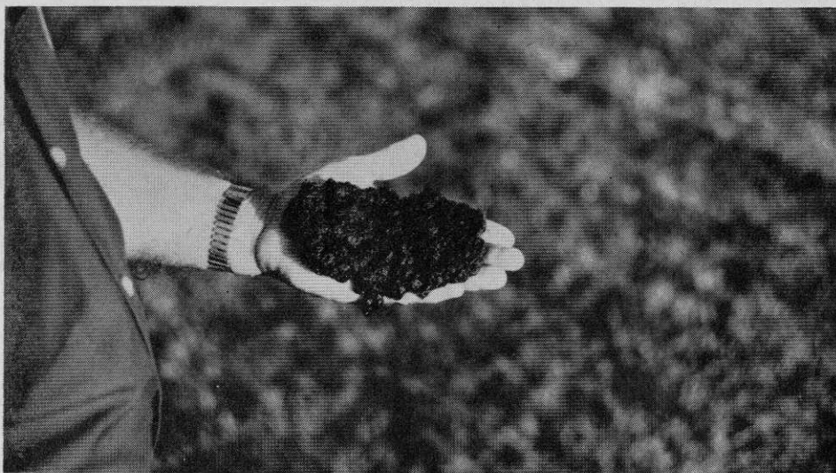
Close-up of mixture of seed and mulch as applied through hydro-seeder to the green.
