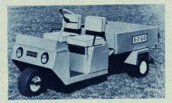
E-Z-GO Car Div., Textron Inc., Augusta, Ga., presents its GT-7 Truck, a new gaspowered, three-wheel, all-steel maintenance vehicle. It features 1500 pound load capacity and one-third larger dump body.
