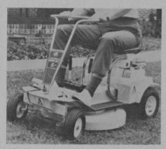
Allis-Chalmers Co., Milwaukee, introduces Mow-Bee 5-hp riding mower. Among its features are: five forward and one reverse speed, individual brake and clutch pedals and swing-away tiller.
