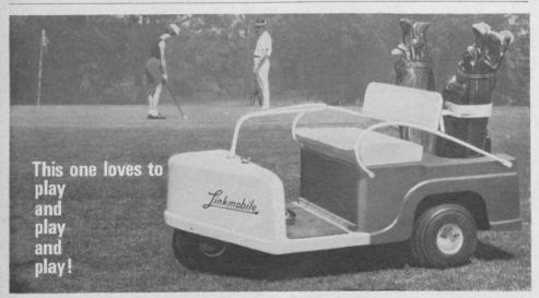
Seldom needs maintenance, this Link-mobile golf car. Simplified design, rugged strength see to that. Make this one easy and fun to drive besides. 8 hp engine levels 35° grades, with speeds to 10 mph. Goes five 18-hole rounds on a 3-gallon tankful of gasoline, with fuel to spare. Heavy-duty Tinkmobile DIVISION, NORTHWESTERN MOTOR CO., FAIRMONT, MINN.
