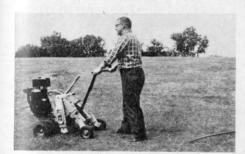
**Sod-Master** has come out with the Pipe Piper, a trencher which lays wire, cable and pipe underground without removing turf.
