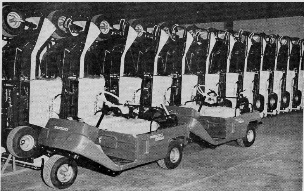
Figure III—Using this method, five golf cars can be stored in an area which would otherwise only accommodate two golf cars.
