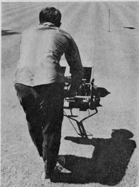
On first longitudinal cut, aim at object on far side of green to insure straight line.
