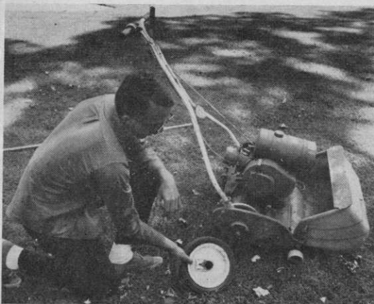
Upon approaching the green, stop below bank, remove transport wheels from mower.
