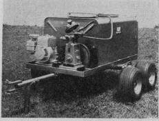
**Root-Lowell Corp.,** Lowell, Mich., has introduced the Turf-Saver Wheel Set, a tire conversion set for heavy-duty sprayers.
