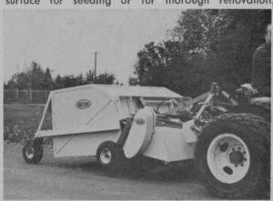
"The Master Verti-Groove and Catch-Master for fast fall renovation—one man cuts and cleans in one operation."
