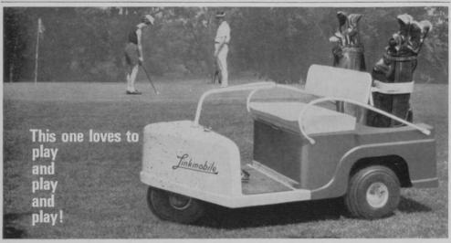
Seldom needs maintenance, this Link-mobile golf car. Simplified design, rugged strength see to that. Make this one easy and fun to drive besides. 8 hp engine levels 35° grades, with speeds to 10 mph. Goes five 18-hole rounds on a 3-gallon tankful of gasoline, with fuel to spare. Heavy-duty
