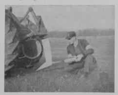
a plow-coulter in front of the arm of the sub-soiler. I can now drain areas with no damage to the turf. The only tell-tale marks are a ½ inch slice through the ground, and a slight heave of the ground of about 1½ inches. This heave will fall to normal after the Spring thaw.
