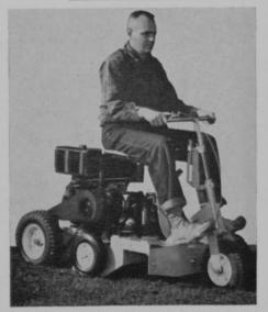
This 32R is a riding rotary manufactured by the Devere-Locke Division of Locke in Racine, Wis. Available with electric starter at extra cost, the Devere-Locke 32R comes equipped with three of its five wheels with pneumatic tires. It weighs 590 lbs.
