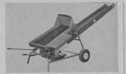
A new machine designed for the preparation and conveying of fine soil mixes is now available from Royer Foundry & Machine Co., Kingston, Pa. This new machine, the POWERscreen 42, is a combination of a vibrating screen desk and elevating conveyor assembled together and operating from a single power source. Power units are available with gasoline or electric motor.
