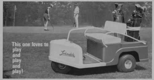
Seldom needs maintenance, this Link-mobile golf car. Simplified design, rugged strength see to that. Make this one easy and fun to drive besides. 8 hp engine levels 35° grades, with speeds to 10 mph. Goes five 18-hole rounds on a 3-gallon tankful of gasoline, with fuel to spare. Heavy-duty
