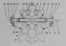
coated shaft sleeves have given better service in many instances than even stainless steel.
