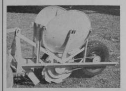
Revolving discs keep sprigs in place for automatic feeding. One man operation.
