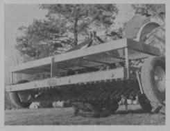
during stress periods when more thorough cultivation is impossible. The unit's action opens the way for movement of water and air and prunes roots to stimulate new growth. It is claimed that the tractor drawn Verti-Slicer doesn't injure turf and makes cleanup unnecessary.
