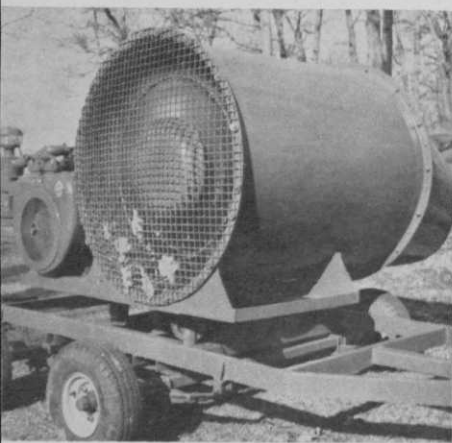
Low slung blower blasts leaves and sprigs and deposits them some 100 feet away. At right is closeup of hydraulic hand brake. Bartlett plans to convert it to a foot-operated brake.
