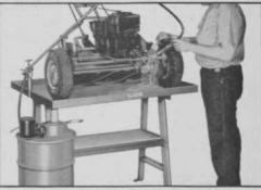
simplex 150 Portable Lapping Machine reconditions any hand, power or gang reel-type mower with lapping compound. Keeps mowers in top condition between sharpening. Couples to either side of mower (gang mowers need not be unhitched). 30 lbs. GE ½ hp. motor with reversing action for quiet, dependable operation.
