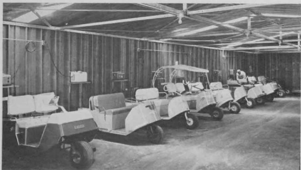
Six skylights help illuminate interior of car storage building at Middletown club. Building has a concrete floor and eight-foot wide overhead door.
