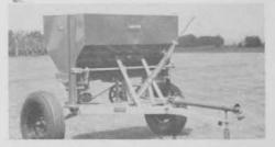
In the new line is the 410 trailer type broadcaster, with 15 cu. ft. hopper, said to be ideal for courses. A modification of the 410 is the 403 "Piggyback" with 15, cu. ft. capacity and 3-point tractor hookup. All Larson models cast spreads up to 50 ft. in width. Complete information on the line can be obtained from L. L. Larson Machine, Inc., Princeville, Ill.
