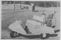
golf cars, manufactured by Tri Powered Corp. of Austin, Tex. This, it is claimed, gives both models positive upbill and downhill driving power that is transmitted through either two-groove or three-groove wedge belt sheaves. TeeBirdies feature tough fiberglas bodies with impregnated color, four large coil springs for automotive type riding and tiller control.
