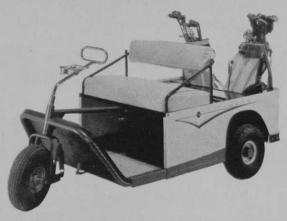
Exciting new body styling designed for comfort and durability. Three point suspension features coil springs with hydraulic shock absorbers plus adjustable anti-roll torsion bar. Direct gear drive, insures highest obtainable efficiency. Up to 54-Holes or more on one battery charge. Bag compartment holds clubs in upright position. Ideal for the private owner—perfect for the rental operator. Only 10% down on Sears Easy Terms—Satisfaction guaranteed or your money back.
