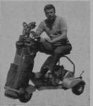
is nicely balanced. It has a 4-cycle, 3 hp Briggs & Stratton gas engine and a 3-qt. tank provides enough fuel for seven hours of average running. An "accelebrake" controls the accelerator and brake through a single pedal. The scooter also has either single- or double-speed range that is selected by a shift lever. Goodyear superrib tires of 10 lb. pressure and powerful front and rear coil springs are said to assure easy riding.
