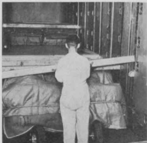
Second deck goes into van. Brackets hold horizontal cross braces onto which a floor is laid. Cars are carefully protected by padding.
