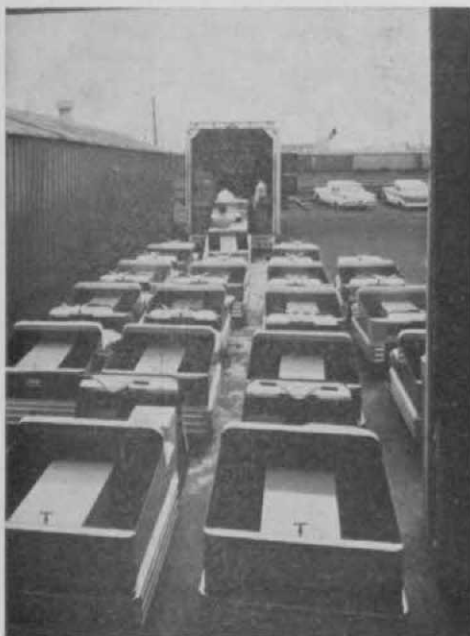
Special van built to accommodate 20 cars is loaded direct from factory door. Cars, of course, enter and leave van under their own power.
