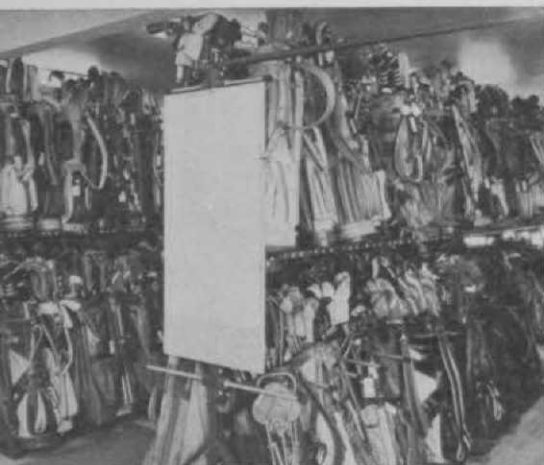
Upright racks save wear and tear on bags, make it easy to get at them. Boards on end of racks hold location index.
