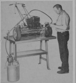
a 12-gauge metal sink sloped to one corner and a separate motor pump unit which clamps to a 5-gal. drum of solvent. The sink supports the largest and heaviest mowers. The motor pump recirculates up to 2 gals. of solvent a minute and dirt and grease are caused to settle in the bottom of the drum. Only clean solvent is picked up and recirculated. There is no spraying or splattering of the liquid. F-R-H's new stand is known as Model 80.
