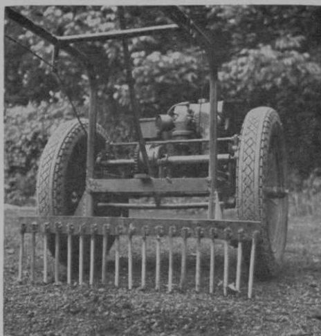
This power driven bunker rake is used by Supt. Nelson Monical at Portage CC, Akron, O. Monical designed the rake. Grau photo
