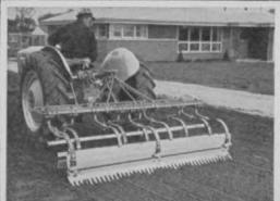
SCARIFIES, GRADES, PULVERIZES, SPREADS, LEVELS, FINISH RAKES
