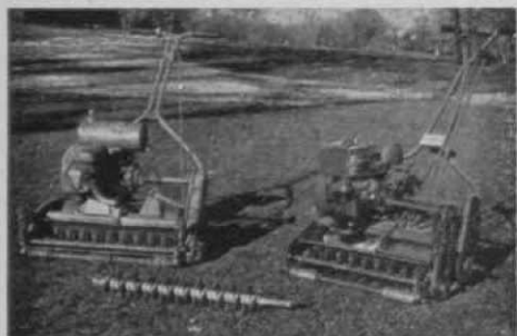
Par Thatcher installed in Toro and Jacobsen greensmowers (Models T, T-1, J)
