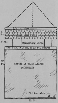
It's a leaf sweeper, which is diagrammed by the ingenious typewriter drawing Shields made for the Mid-Atlantic GCSA Turf Letter.
