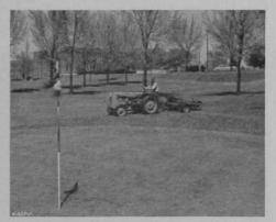
Mowing 350 acres of fairways and park land at Wood, Wis., has been reduced to a minimum by teaming up the Veteran's Administration's two Allis-Chalmers Model IB tractors. Operators of equipment report efficient handling and flexibility of IB tractors provides short-turn radius reducing mowing time around trees, undergrowth and other stationary objects.
