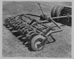
with saw-toothed knives, adjustable in penetrating depth from 2-3-4 inches. These saw-tooth knives are shaped so as to perform a definite slicing action in controlling long step grasses and cutting endless number of slits 2 in. long in turf without tearing the surface.
