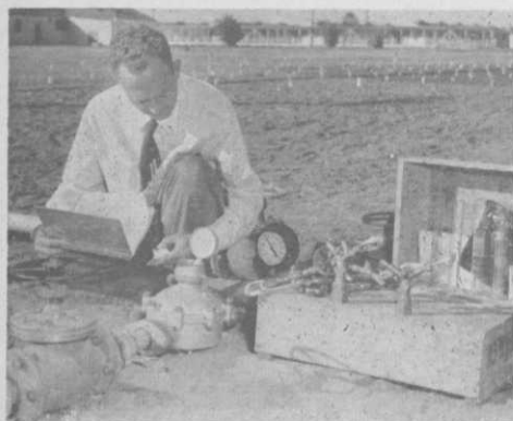
H. M. Clark, Buckner chief eng., clocks flow of water thru test pipe at irrigation school. Water distribution is measured from cans in background.
