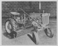
Mott Hammer-Knife mower for tough rough and brush is new attachment approved for use with International Farmall "Cub" tractor.
