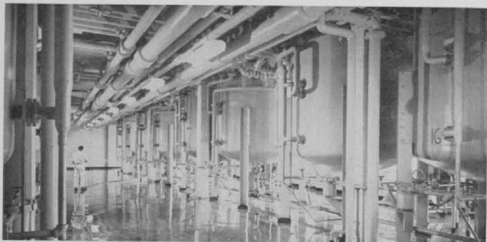
Battery of fermentors (as seen from below) used in the manufacture of antibiotics.
