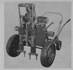
stronger one-piece cast ram housing, more positive chain and belt alignment, and uniball joints on the walking beam are included in the improvements. Change-over kits are available for all previous models. Full particulars from the manufacturer.
