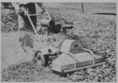
pulverizes them and blows the mulch back on the turf or into a bag. The 6 hp model, shown above, is self propelled, cleans 3 ft. swath. A larger, 25 hp tractor drawn model cleans a 6½ ft. swath. Full particulars from the company.
