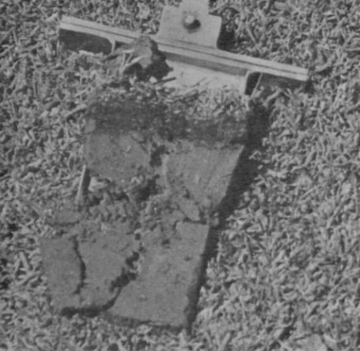
Fairway soil sample taken prior to aerification program; note thatch formation at surface.
