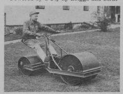
ton engine, the roller is operated by a tiller-type steering bar and a single lever for both forward and reverse.
