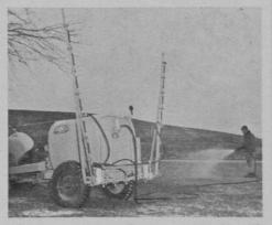
All sprayers completely equipped, with adjustable tread and axle clearance adjustment, ready for use with boom controls on sprayer when specified. Accompanying photo shows boom in position for transporting from one area of course to another when not in use.
