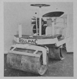
Soilaire Industries, 1200 Second ave., S., Minneapolis 3, Minn., has its new Rollpac power roller in production. The roller is of all-steel construction; built of formed steel channels and plates. Engine is Briggs & Stratton, 5 hp. Clutch is twin disc. Toro planetary transmission is used. Hollow rollers are built of 3/16 in. plate. There is a double seat position for forward or reverse operation. Weight can be varied from 720 lbs. light to 1725 lbs. loaded with operator.
