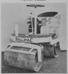
Soilaire Industries, 1200 Second ave., S., Minneapolis 3, Minn., has its new Rollpac power roller in production. The roller is of all-steel construction; built of formed steel channels and plates. Engine is Briggs & Stratton, 5 hp. Clutch is twin disc. Toro planetary transmission is used. Hollow rollers are built of 3/16 in. plate. There is a double seat position for forward or reverse operation. Weight can be varied from 720 lbs. light to 1725 lbs. loaded with operator.
